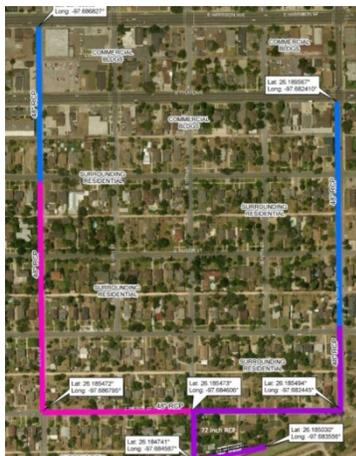
The 9<sup>th</sup> and 13<sup>th</sup> Street Drainage Improvement Project will also help improve storm water run-off. These improvements were identified in the City's 2008 Master Drainage Plan. This is a large project that calls for the removal of the existing storm sewer drain pipes and replacing them with 48-inch reinforced concrete pipes. Fourteen manholes and 52 inlets will also have to be removed and replaced.
