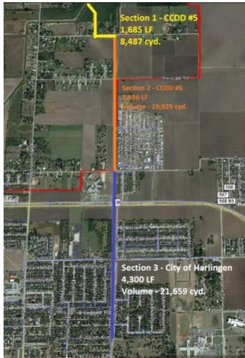
This ditch serves a large area that includes several subdivisions, a high school, a fire station, sanitary sewer lift stations, commercial development, and undeveloped land currently used for agriculture. The scope of the work here includes widening the ditch and increasing the size of one culvert crossing.
