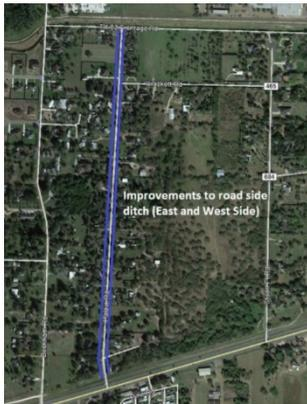
Some driveway culverts will need to be removed but will be rebuilt at a new slope that will allow for a positive flow of storm water.
